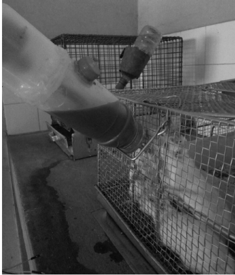
Figure 10: Photo of small animals feeding on the auto-homogenize feeding bottle
